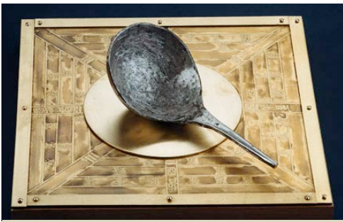
Early Chinese compass with a lodestone spoon handle that pointed north
